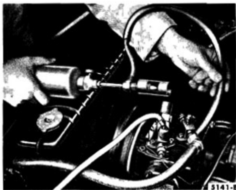
Fig. 32—Using Leak Detector
