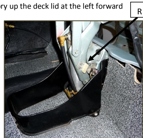
RIGHT HINGE – The right rear deck hinge and deck “open” switch, (R) are seen here. See figure II in this article.
