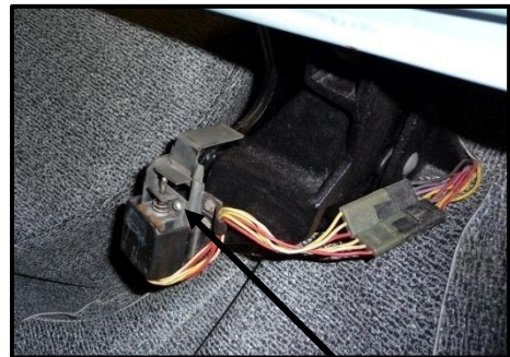
TOP DOWN – The right hinge “Down” switch is located next to the spare tire.
